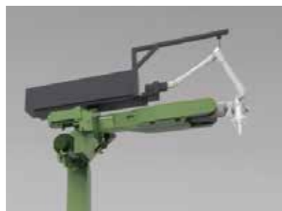
导光臂悬吊方案 Ceiling-mounted Beam Delivery Solution
